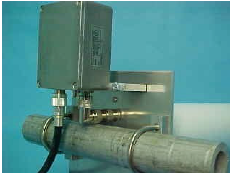
2400-144RX mounted to a DSH 12-27 antenna.
